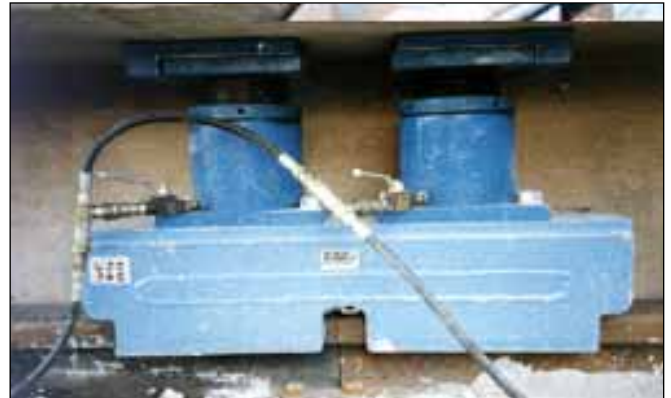
Above and Below: The vertical jacking facility provides a hydro-cushion support and controls final positioning.
