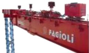
The Elevator System is a specially designed system able to lift and skid items up to several thousand tons
