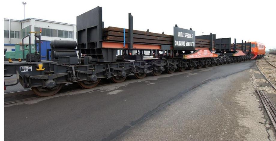
**48** axles lines (24 x24) used for the test process of High Speed Rail Line, loaded with billets weighing about 1,100 ton
