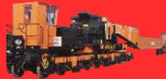
Rail Wagons for heavy rail transports with capacity up to 500 ton. Different possible configurations with rail cars up to 32 axle lines
