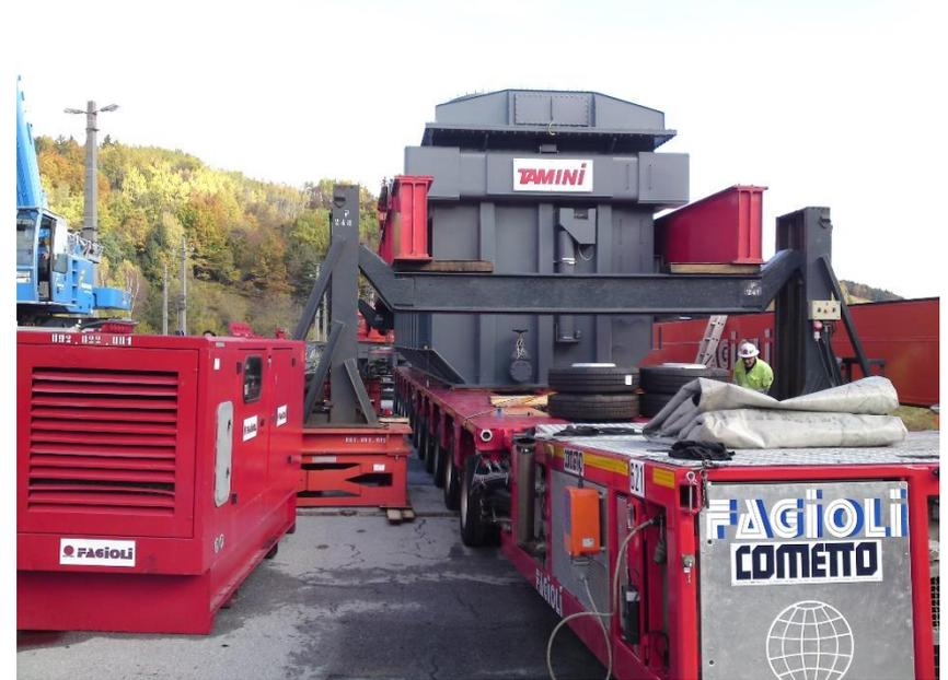
Once arrived at Arnoldstein, the support structure was removed and the trafo was skidded with the support of rollers and beams. The item was lifted with screw jacks and positioned onto 12 axle lines modular trailers. The challenge for the last leg of the journey was not the distance between the railway and the power station (almost 3 kms) but how steep was the road: a slope of 15%.
