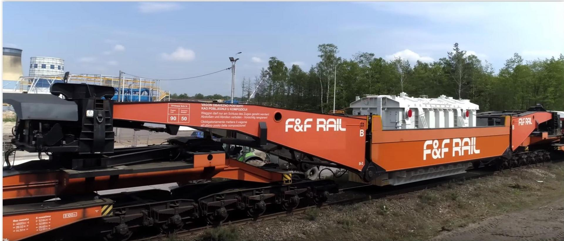
Rail transport of **190 tons** transformer.
