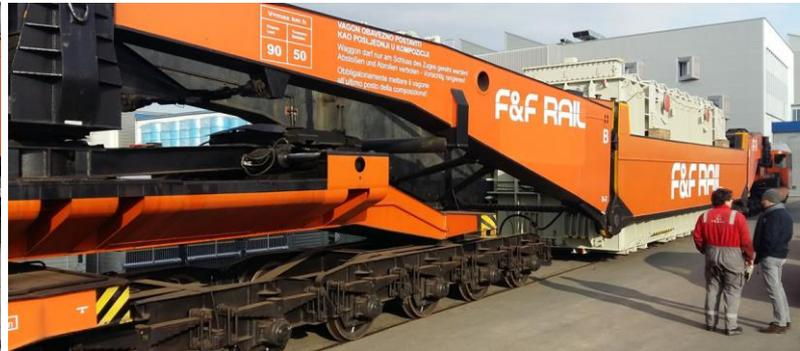
Rail transport of No. 2 Transformers (140 ton /220 ton)
