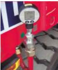
Fagioli calibrated digital pressure gauges could be installed onto SPMTs and Skid Shoes for accurate weighing operations
