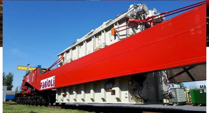
Rail transport of **150 tons** transformer.
