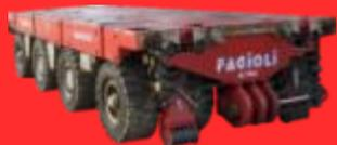
Dedicated trailers for the heavy transport. 4-5-6 axle lines modular trailers with capacity up to 60 ton per axle line
