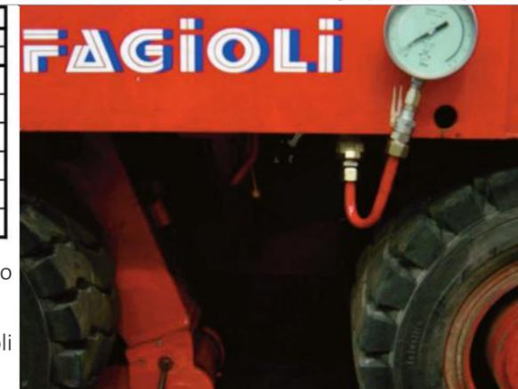
Above: Drawing example of the positioning of manometers onto SPMTs and technical schedule for the collection of weighing data. Picture on the right: Detail of manometer positioned onto Fagioli SPMT trailers.
