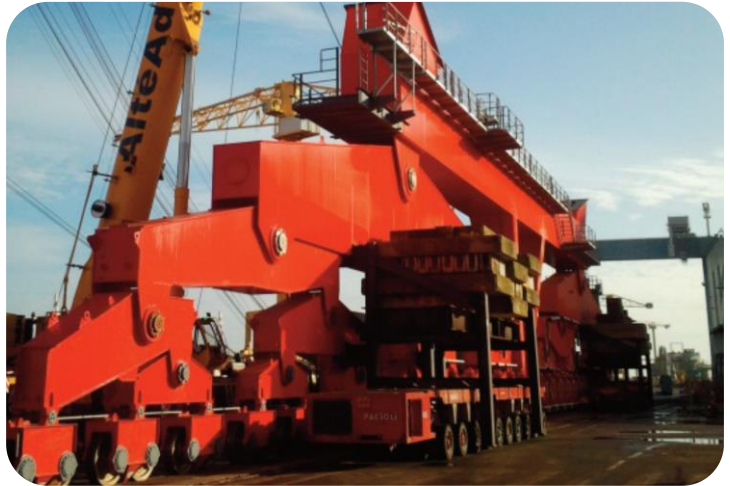
Above: Bogey with SPMTs support (Stage 6)
